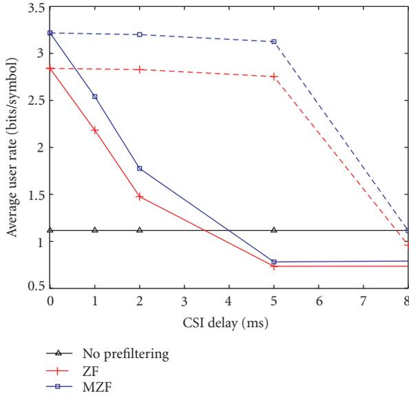
FIGURE 7: Average rate per user versus CSI delay, with MMSE prediction (dashed lines) and without MMSE prediction (solid lines) (SNR = 10 dB,  $M = 3$ ,  $N = 3$ , channel based on model in (20),  $f_c = 2$  GHz,  $v = 30$  kmph).
