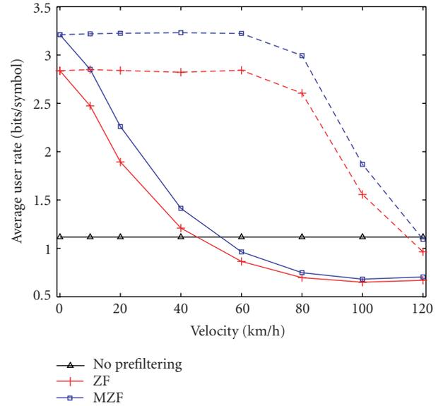
FIGURE 8: Average rate per user versus terminal velocity, with MMSE prediction (dashed lines) and without MMSE prediction (solid lines) (SNR = 10 dB,  $M = 3$ ,  $N = 3$ , channel based on model in (20),  $f_c = 2$  GHz,  $\tau = 2$  milliseconds).
